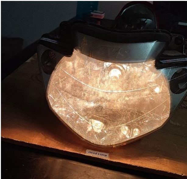
Figure 6 Halogen lamp at High Beam
