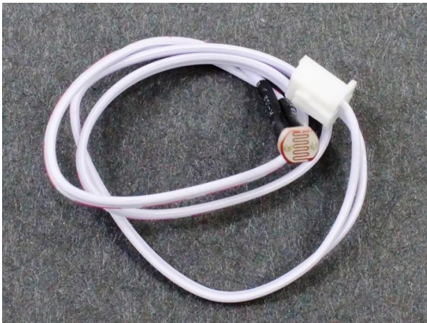
Figure 2 LDR Sensor of light sensitive Relay module
