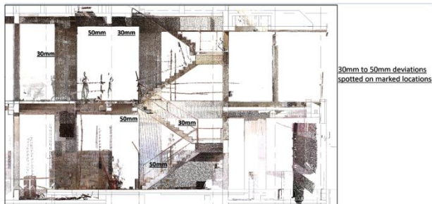
Figure 5 Deviation identification by comparing Scan to BIM model & design
